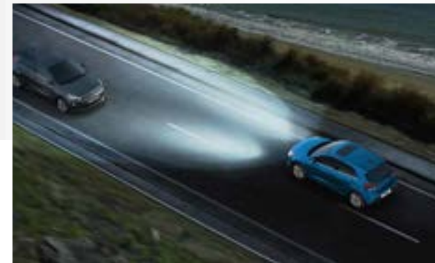
High Beam Assist Cameras embedded in the windscreen detect oncoming vehicles at night and automatically switch to a low beam to avoid dazzling other drivers. Once the oncoming vehicle has passed, the high beam is switched back on.
