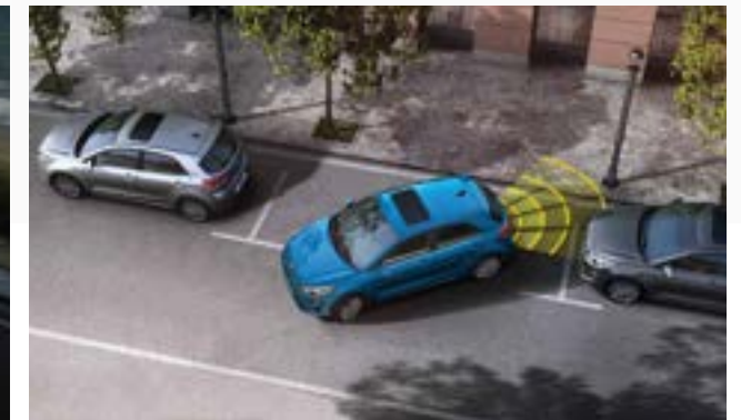
Reverse Parking Distance Warning (PDW) with Switch On/Switch Off button Ideal for confident parking, PDW uses ultrasonic sensors mounted on the rear bumpers to warn of any obstacles in front or behind when manoeuvring into a parking space. The audible beeps can be switched on or off.
