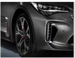
Front bumper with integrated air curtain The Stinger's breathtaking front serves a clear purpose; the front bumper's integrated air curtain helps manage airflow, reduce drag and direct cooling air to the radiator and front brakes. Equally, the lower apertures direct airflow to the wheel wells, which reduces drag and helps cool the brakes. Aside from fuel savings and noise reduction, the front design also contributes to the car's stability. Please note that the Brembo brakes are only with the GT.
