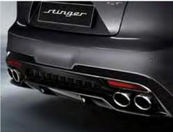
Rear integrated diffuser An integrated diffuser panel under the rear bumper helps control airflow and prevents the dual exhaust pipes from creating drag under the car. It pays homage to racing diffusers which lower the turbulence that can occur when low-pressure air under the car meets higher pressure ambient air.
