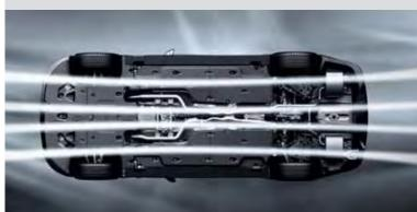
**Multiple undercovers and aerodynamic effects** While the aerodynamic aspects of the silhouette are plain to see, the Stinger also boasts vital drag reduction features that improve airflow underneath the car. It uses a system of sturdy undercovers, below the engine and transmission, each side of the cabin, and each side of the rear suspension. These covers reduce the flow resistance on the underside of the body when travelling at higher speeds.
